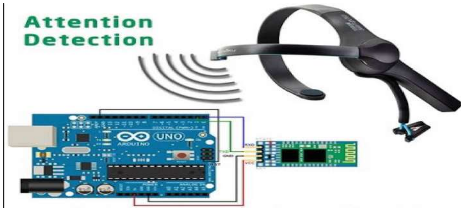
Fig. 5. Shows the interfacing of Arduino with Mindwave headset
